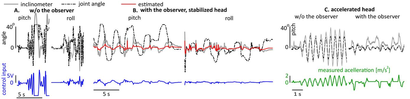
Fig. 4. Experimental results. **A:** stabilization based on direct roll and pitch measurements from the inclinometer. **B:** stabilization based on the estimated head's orientation. The system was stable. **C:** head stabilization during horizontal acceleration based on direct inclinometer measurements (left panel) and based on state estimation (right panel).
