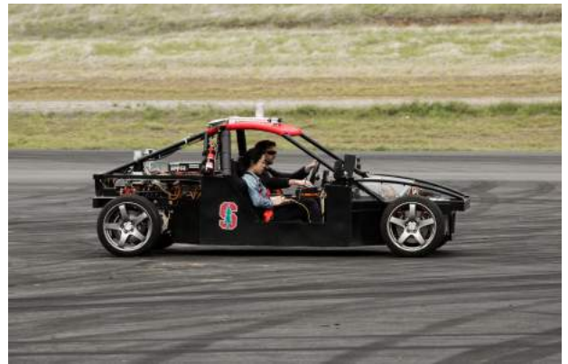
(b) Outdoor experiments using X1 — a drive-by-wire research vehicle at Thunderhill Raceway Park, CA
